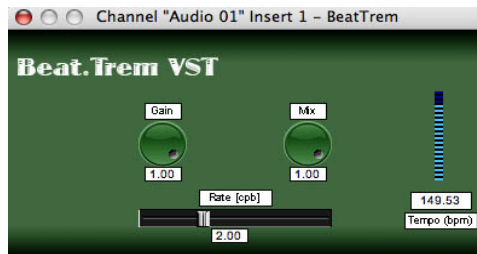
Figure 1: A Beat-Synchronous Tremolo effect implemented as a VST Plug-in. The rate is controlled by the number of cycles per beat (CPB).
